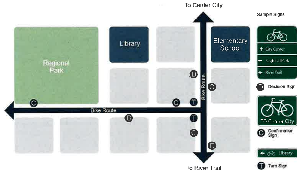
Figure 12 Typical Locations for Wayfinding Signage
